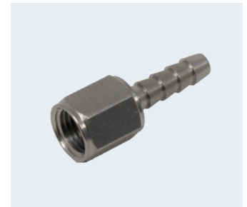
P/N 17697: Barbed Hose Fitting—1/4" HB x 1/4—18FPT—SS
